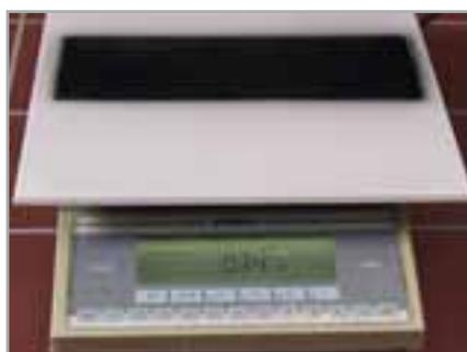
Fig. 2 Weighing of tile with test soil
