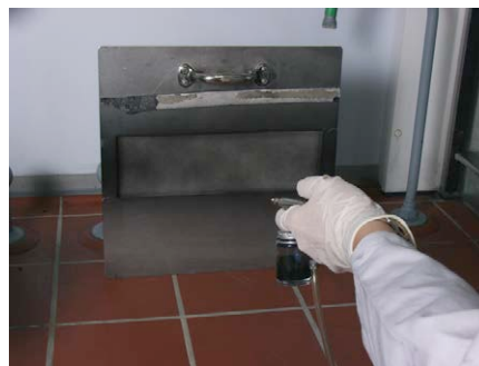
Fig. 1 Application of test soil, using a stencil. (Source: Werner & Mertz GmbH, Mainz)
