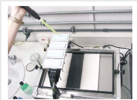
Fig.3 Application of test cleaner. (Source: Werner & Mertz GmbH, Mainz)
