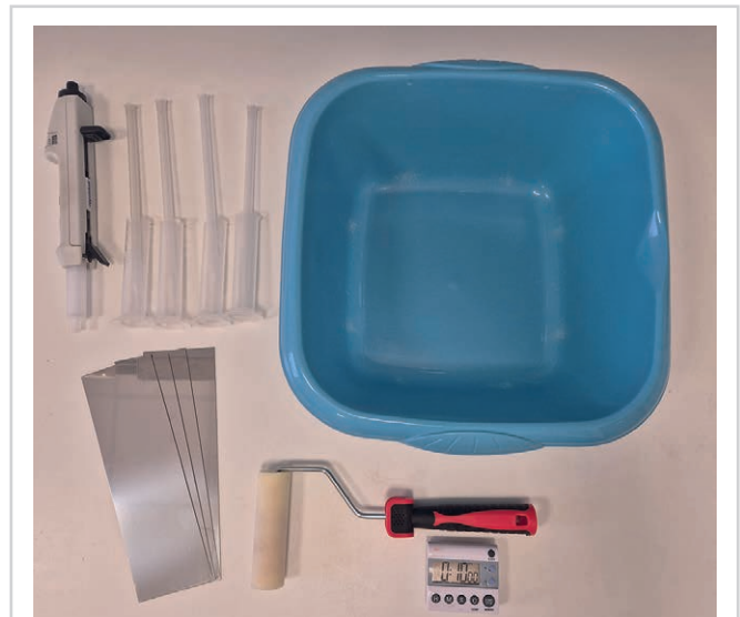
Fig. 2 Extract of the required items for the test method: stainless-steel plates, pipette, syringes, paint roller, timer and plastic tub.
