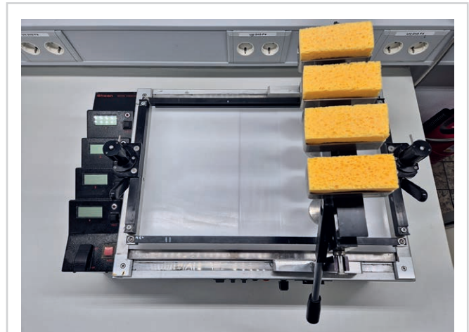
Fig. 1 Multi-track scrub tester with sponge brackets, shown here is the Sheen PG 903 model, for use in wiping and scrubbing tests.
