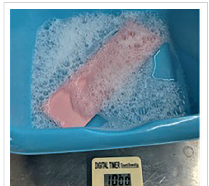
Fig. 6 Soaking of a soiled stainless-steel tile in the soaking solution for 10 Minutes.
